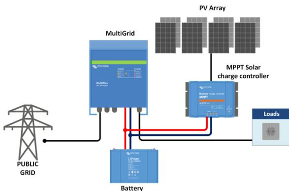
**Grid in-line topology with MPPT solar charge controller**
