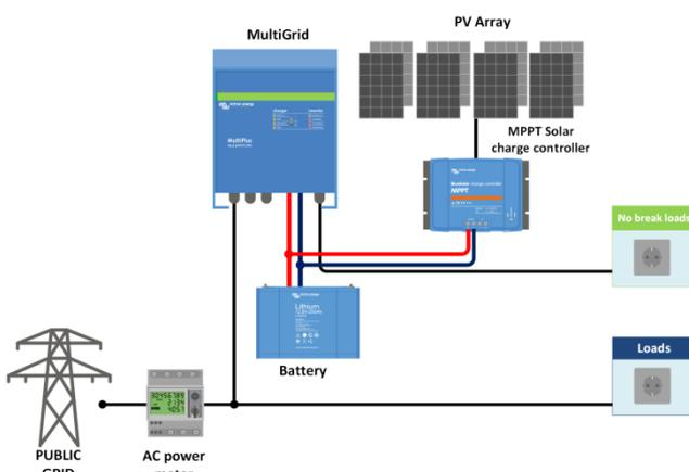
**Grid parallel topology with MPPT solar charge controller**
