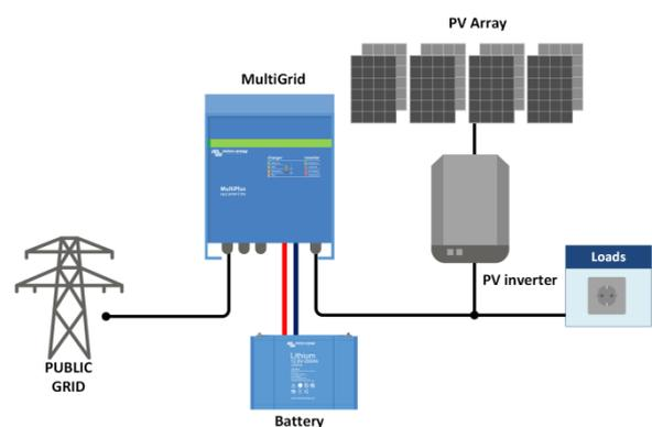
**Grid in-line topology with PV inverter**
