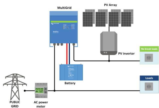
**Grid parallel topology with PV inverter**
