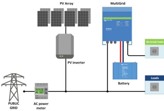
**Grid parallel topology with PV inverter**
